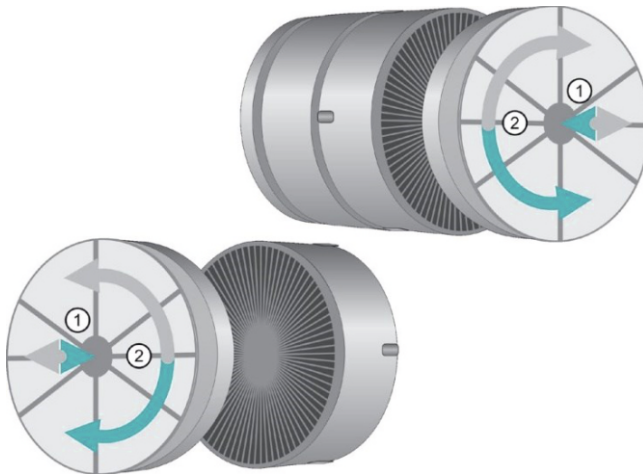
Pic. 14 Carbon filter installation
